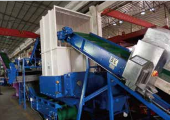
单轴撕碎机WTF40120 配磁选生产线 Single shaft shredder WTF40120 with Magnetic separation
