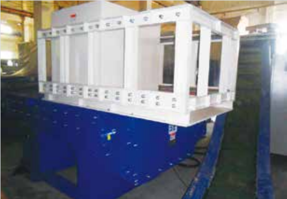
管材撕碎机WTP4080破碎线 Pipe shredding system WTP4080
