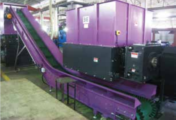
单轴撕碎机WT40150 与破碎机PC52120生产线 Single shaft shredder WT40150 with Granulator PC52120
